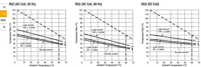
The above temperature rise curves show the characteristics when 100% the rated coil voltage is applied. The heat resistance of the coil is 120°C. The slant dashed line indicates the allowable temperature rise for the coil at different ambient temperatures.
