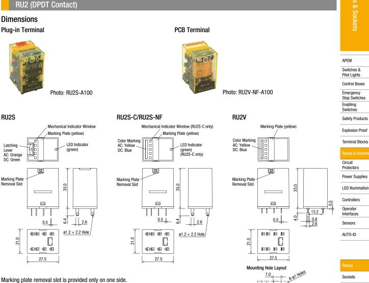
Marking plate removal slot is provided only on one side. Insert a flat screwdriver into the slot to remove the marking plate.
