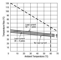
The above temperature rise curves show the characteristics when 100% the rated coil voltage is applied. Load current  $6A \times 2$  poles is for the RU4 only.
